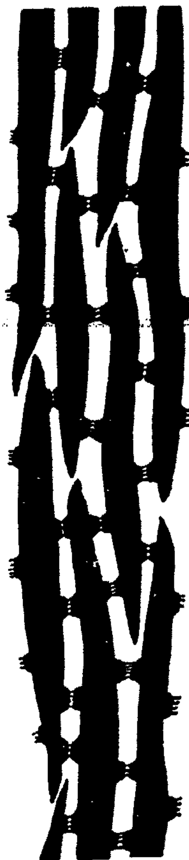
FIG. 1 Simplified diagrammatic representation of the capillary path through wood showing the manner in which the fiber cavities are connected through the pores of the pit membranes.
